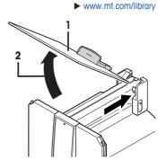
2 Insert the liquid kit (1), pull 2 levers (2) towards you and slide liquid kit onto the rack.
