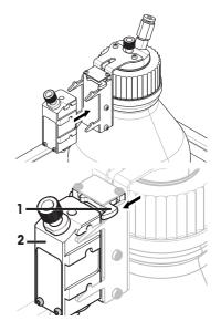
2 To remove liquid dosing head from the liquid dosing head support, pull the catch (1) to the front and remove liquid dosing head (2).
