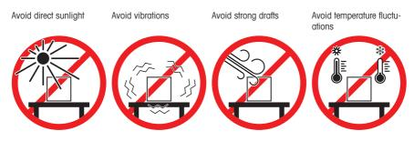
Sufficient spacing for balances: > 15 cm all around the instrument Take into account the environmental conditions. See "Technical Data".
