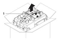
Open the lifting strap (1) and remove the User Manual (2).
