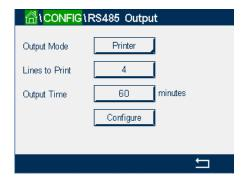
The Printer option allows configuring the M800 RS485 output to send data to a suitable printer. The printer output may be configured to print up to 6 configured measurements on separate lines, for each available sensor input, including pulsed input channels. At each print cycle, the output will include a header line with data and time based on the M800 internal clock, and one line for each configured measurement including channel, measurement descriptor, measurement value and unit of measure.
