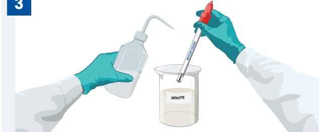
Rinse the sensor with deionized water (tap water is OK if no deionized water is available).
