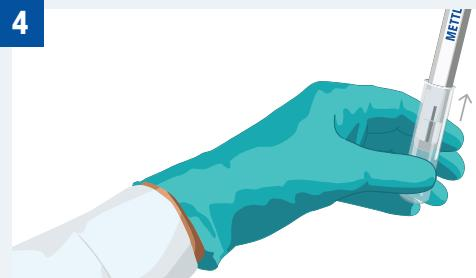
Fill the watering cap with fresh 3M KCL solution and attach it to the sensor. Take the sensor to your maintenance workplace.
