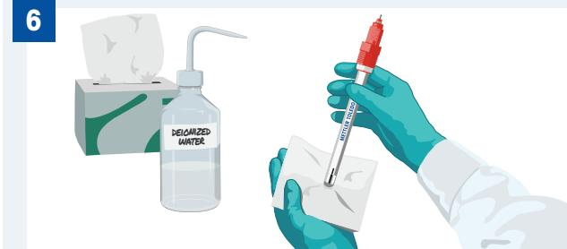
Once clean, rinse the sensor with deionized water and gently pat it dry with Kimwipes or an equivalent. (Do not wipe the sensor as this can induce an electrostatic charge which will affect measurement.)
