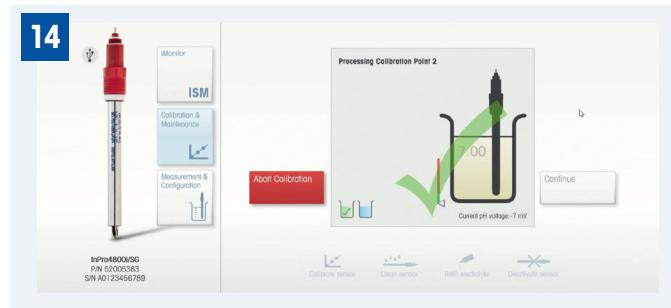
Wait until you see the checkmark to confirm the first buffer reading.
