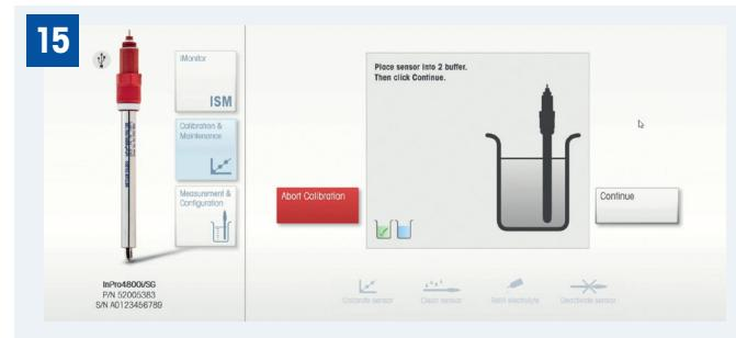
Rinse the sensor with deionized water and pat dry (see step 6) before placing the sensor in the next buffer. Click "Continue" and follow the on-screen instructions. Wait for the checkmark and successful calibration.
