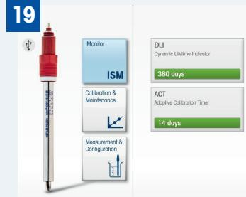
Display the predictive diagnostics, DLI and ACT, to show when the next calibration or sensor exchange is due.
