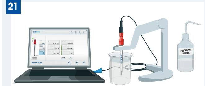
Click "Measurement & Configuration" and place the sensor in pH 7.0 buffer for verification. If the displayed value is not correct, repeat the process from step 13. If the displayed value is correct, rinse the sensor with deionized water and pat dry.
