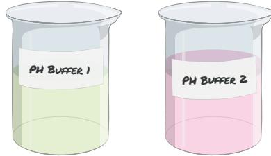
Pour each of the required calibration buffers into separate, clean beakers. (Never place the sensor into the buffer bottle as this can contaminate the buffer, even if the sensor has been cleaned.)
