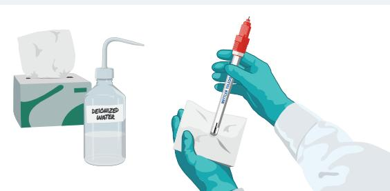
Rinse the sensor with deionized water and pat dry.
