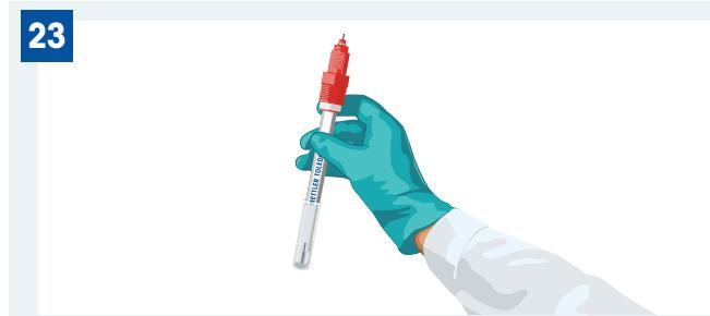
Fill a clean watering cap with new 3M KCl storage solution. Cap the sensor such that its membrane tip and diaphragm are totally submerged.
