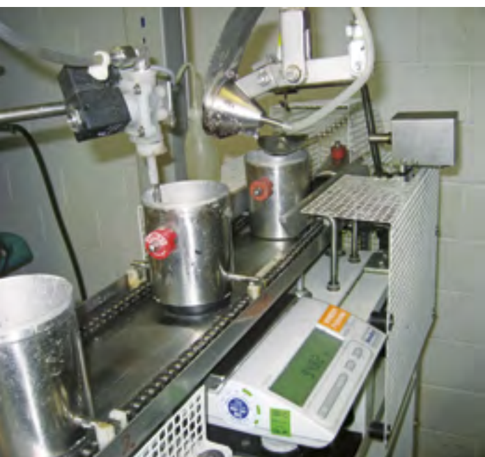
A METTLER TOLEDO precision balance is integrated into an automatic sugar content determination process.
