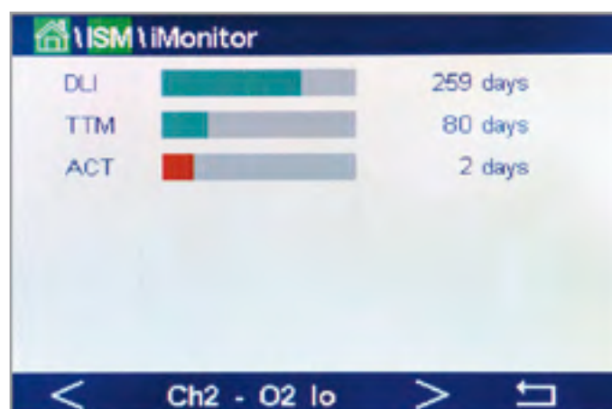
Figure 2: ISM advanced diagnostics with calibration, maintenance, and parts replacement reminders
