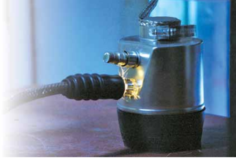
POWERCELL PDX load cell under laboratory testing of a simulated lightning strike.
