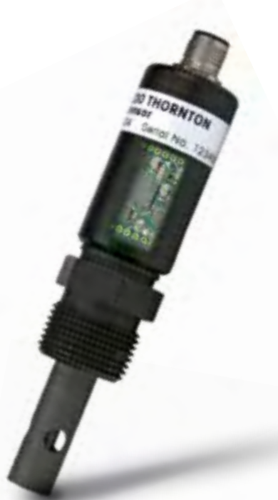
Figure 2 – UniCond conductivity sensor with cut-away view of internal measuring, digital conversion and memory circuits
