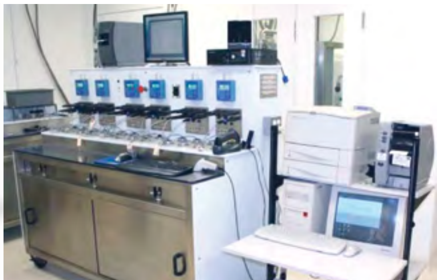
Figure 3 – Automated conductivity/resistivity sensor calibration facility
