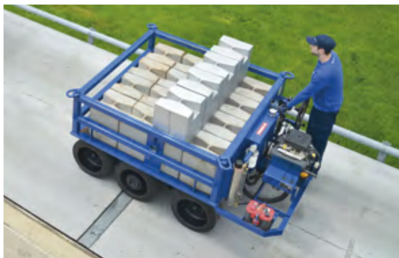
Replacing a conventional load cell, cable, or junction box requires time-consuming recalibration with heavy test weights.
