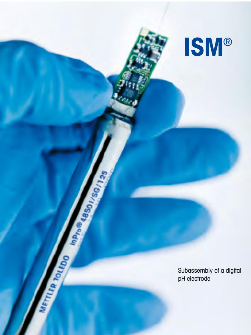
Subassembly of a digital pH electrode
