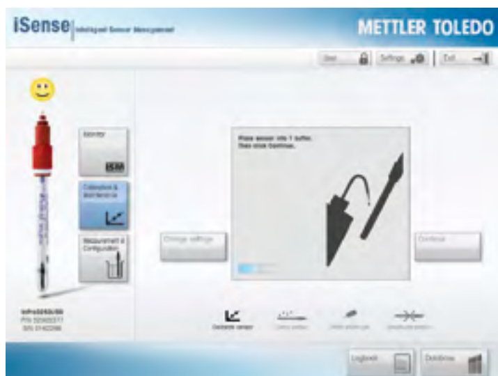
On-screen animations guide you through maintenance procedures, helping to ensure proper handling.
