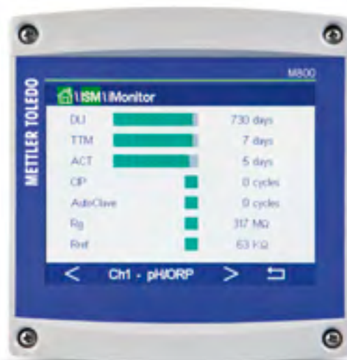
M800 transmitter showing iMonitor sensor diagnostics utility.
