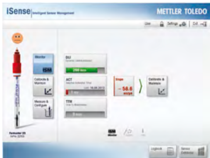
The smiley provides at-a-glance notification of sensor "health". Diagnostics show that this sensor needs calibrated.
