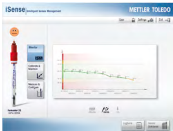
The Sensor History feature allows you to see how a sensor has been affected by process exposure over time, assisting with maintenance planning.
