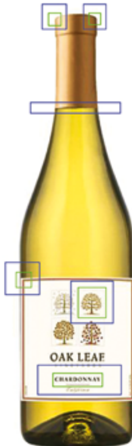
Vision inspection systems on the production line at The Wine Group, ensuring labels are straight and legible, seals are safe and secure, and that bottles are filled accurately.
