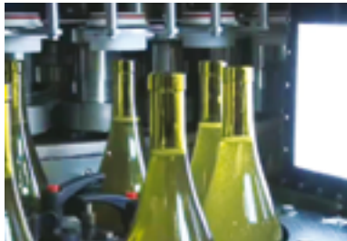
Vision inspection systems on the production line at The Wine Group, ensuring labels are straight and legible, seals are safe and secure, and that bottles are filled accurately.
