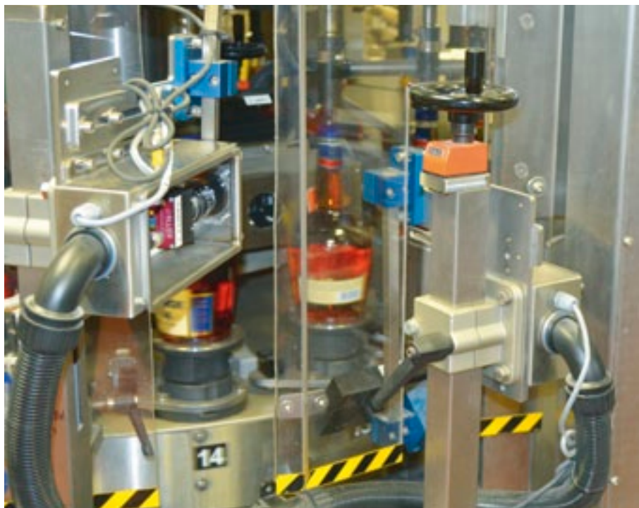
The 4-camera vision inspection solution inspects for proper cap seal & fill level, and correctness of neck, front and back labels on un-oriented glass bottles.
