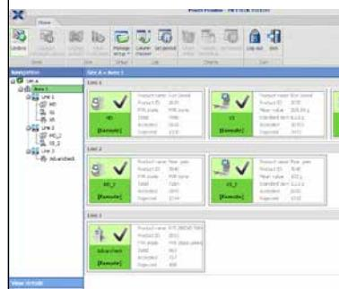
An easy to read dashboard gives a condensed overview of the status and production figures of each inspection device.
