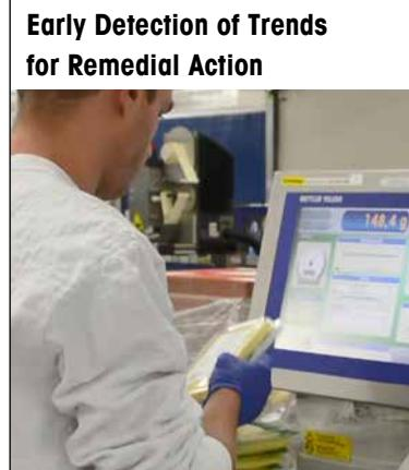
When non-conforming products are detected, ProdX will help to identify trends and instigate preventive action where necessary to prevent recurrences.
