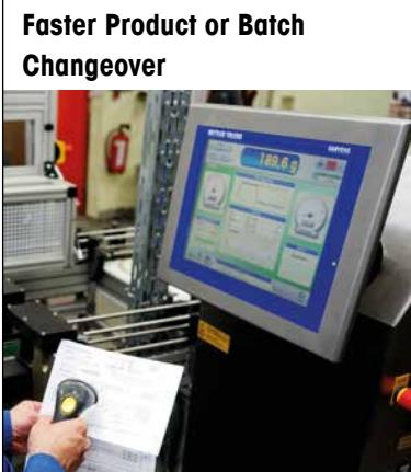
With ProdX, product or batch changes can be performed from a single point for all inspection devices in a line, making changeovers quicker and less
