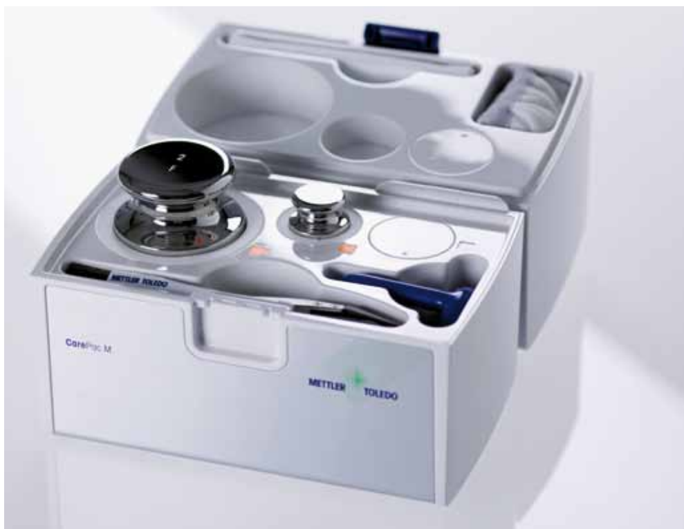
CarePacs® include tweezers, gloves and other accessories for professional weight handling.
