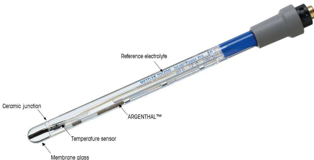
Fig. 2 A combination pH electrode
