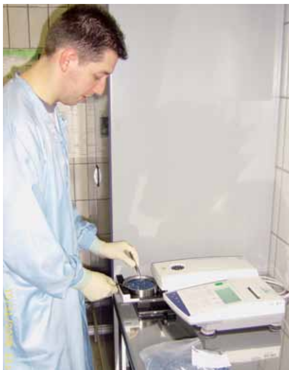
A lab technician of Karl Kufner tests plastic parts with HR83.
