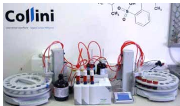
Figure 1: The Titration Excellence system titrates nickel and hypophosphite in parallel including sample preparation.
