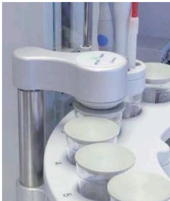
Figure 4: CoverUp™ removes the lid immediately before titration and closes the titration beaker again immediately afterwards. This prevents unpleasant vapors from escaping.
