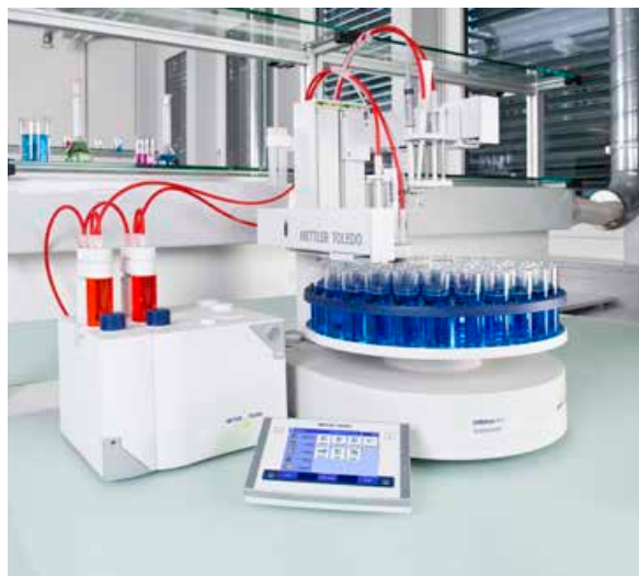
Figure 5: Titrator Excellence with new InMotion sample changer
