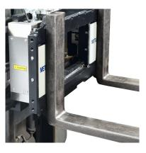
System protection The robust design protects internal components from knocks, bumps and even crashes. If the forks tilt too far to safely weigh, the operator is alerted to the problem.
