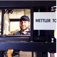
A visibility window placed at the center of the weighing carriage allows the operator to position, load and transport goods safely while maintaining optimal productivity.
