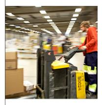
One-step weighing with a forklift eliminates the need to transport loads to and from a floor scale. Speed up the handling process by weighing onboard. Weight data is automatically transferred.
