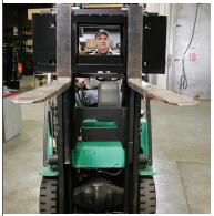
The center of the weighing carriage is open, making it easy for the operator to see loads, position forks for lifting and stay out of the way of other forklift traffic.
