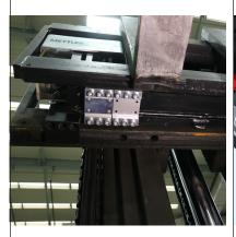
Sometimes fork height becomes uneven as a result of wear and tear. Angular compensation maintains accuracy regardless of the height of the two forks.
