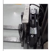
The unique three-point suspension holds calibration for up to twelve months with no need for recalibration. This reduces the expense and inconvenience associated with frequent readjustment.
