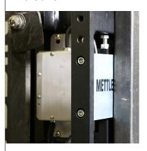
The robust design protects internal components from knocks, bumps and even crashes. If the forks tilt too far to safely weigh, the scale terminal alerts the operator to the problem.
