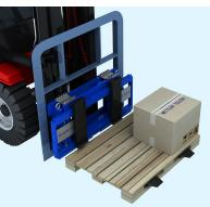
The corner adjustment function allows shipments to be accurately weighed, regardless of where goods are placed on the pallet.
