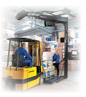
Because the CSN840 can interface with any existing system, Southeastern's computer system can automatically update freight bills with the cubic feet of the total shipment and create a Weighing and Inspection Certificate to document the length, width, height and cubic feet of each piece measured in the shipment. The entire process from measurement to documentation takes less than 10 seconds to complete.
