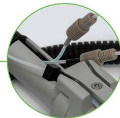
To rinse the tubes in the probe shaft, connect the syringe, the adapter and the tube provided in the EasySampler Pump Rinsing Set to one of the tubes leading to the probe shaft. Place the other end into a vessel and flush solvent through it.
