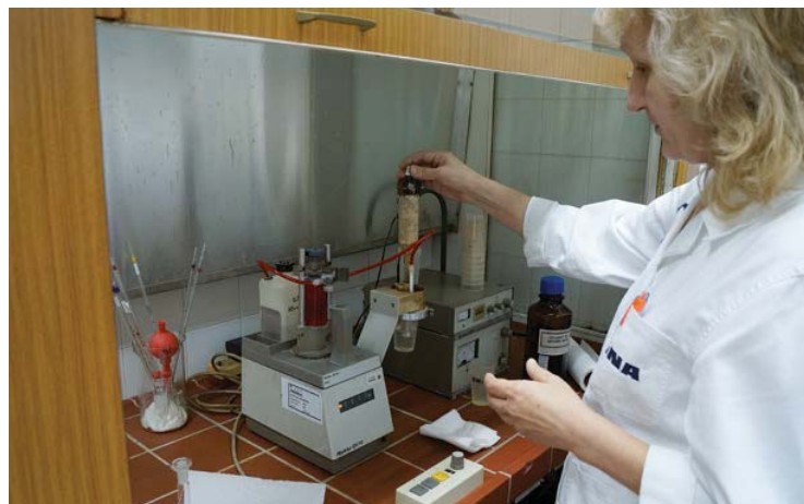
Figure 2: Bromine number determination with the DV10/DK11 titrator system developed at METTLER TOLEDO 40 years ago.
