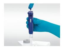
Set the pipette to its nominal volume, then, using deionized water, pipette that volume into SmartCheck's vessel.
