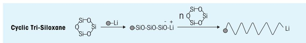
**Figure 2.** Silicone production based on precise polymerization
