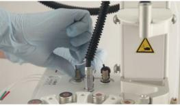
2 Fix the needle in place with the knurled screw.
