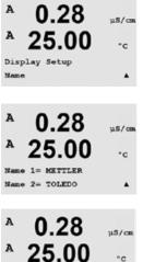
This menu allows for the configuration of an alpha-numeric name which is displayed in the first 9 characters on lines 3 and 4 of the display. The default is nothing (blank).
