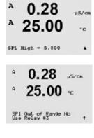
R3 Delay = 010 secon R3 Hysteresis = 05 % Depending on the defined setpoint type, this screen provides the option to adjust the values for the setpoint(s).
