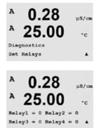
The Set OC diagnostic menu allows to open or close each OC manually. To access OC and 6, press [ENTER].
