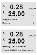
If Memory is selected then the transmitter will perform a RAM and ROM memory test. Test patterns will be written to and read from all RAM memory locations. The ROM checksum will be recalculated and compared to the value stored in the ROM.
