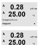
Key press =(MENU ) Press ENTER to Continue For keypad diagnostics, the display will indicate which key is pressed. Pressing [ENTER] will return the transmitter to the normal measuring mode.
