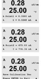
Enter the value for Point 1, in milliamps, of the current source connected to the input. The second display line will show the measured current. Press [ENTER] to begin the calibration process.
