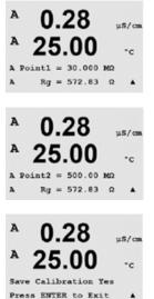
Enter the value for Point 1 of the calibration according to the resistor connected across the pH glass electrode measuring input. Press [ENTER] to begin the calibration process.
