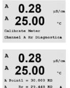
Rr diagnostic is performed as a two point calibration. Navigate to the Calibrate Meter screen and select Channel A and Rr Diagnostic.
