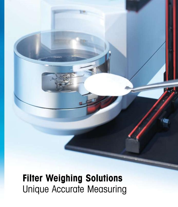
Excellence Balances equipped with a Filter Weighing Kit provide a state-of-the-art solution for emissions determination. The METTLER TOLEDO measurement system enables fast and accurate weight determination down to 0.1  $\mu$ g, meeting strict automotive and environmental requirements.
