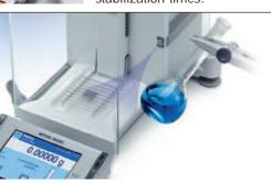
Antistatic kit for XP analytical balances The fully integrable ionizer generates positive and negative ions which immediately eliminate disruptive electrostatic charge.
