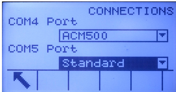
Figure 3-12: COM4 Connection Configured for ACM500
