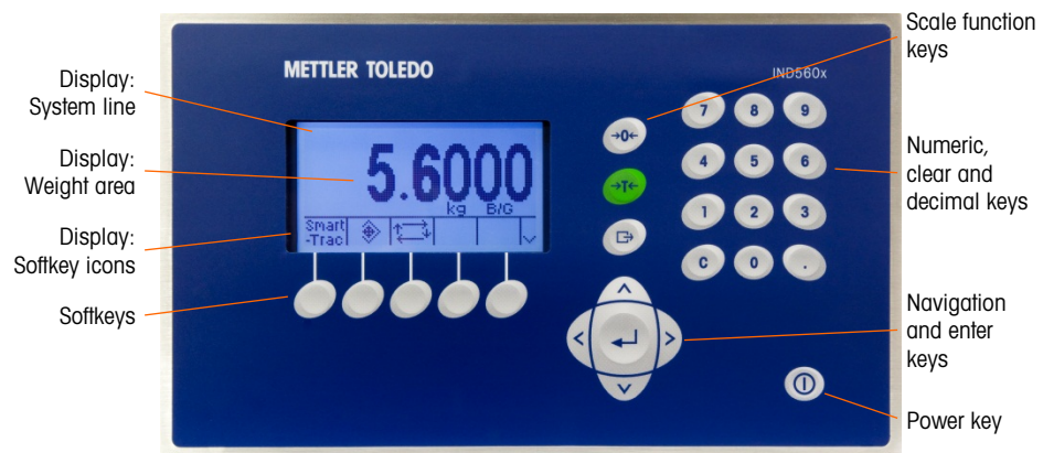
Figure 1-9: The IND560x Display and Keyboard Layout
