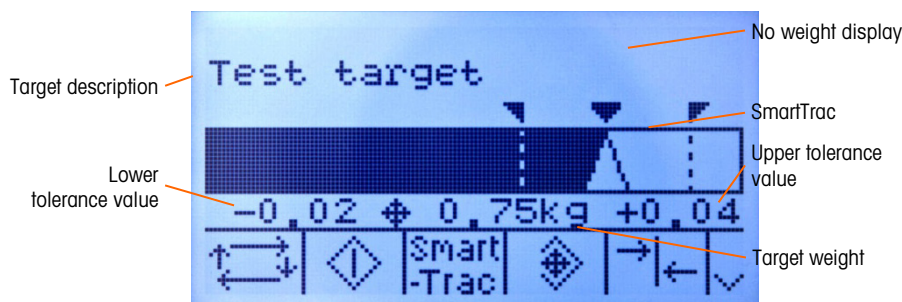
Figure 2-15: Material Transfer SmartTrac, Large
