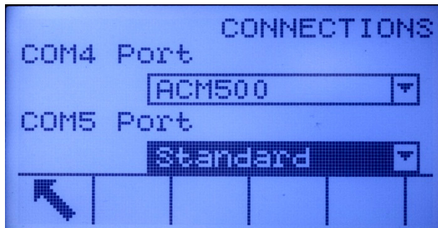
Figure 3-19: COM4 and COM5 Setup
