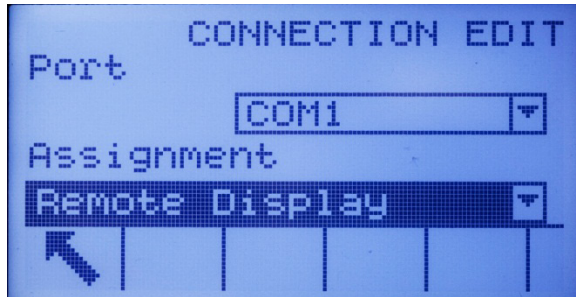
Figure 3-11: COM1 Connection Configured for Remote Operation
