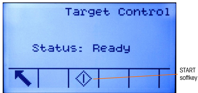
Figure 2-10: Example of Ready State in Target Control
