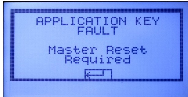
Figure 4-1: Application Key Fault Message
