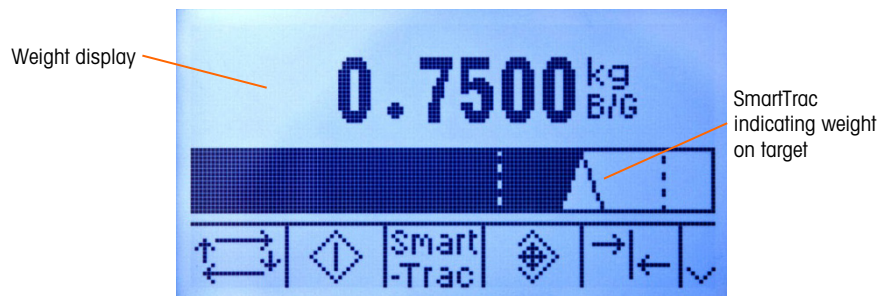
Figure 2-13: Material Transfer SmartTrac, Small
