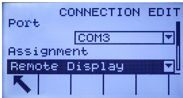
Figure 3-13: COM2/COM3 Connection Configured for Remote Operation
