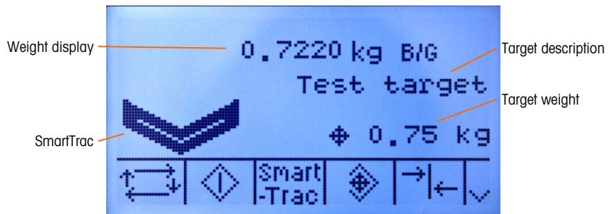
Figure 2-19: Over/Under Display, Medium
