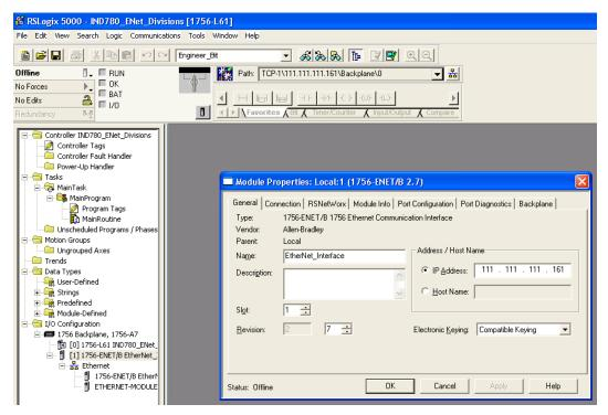
Figure 5-16: EtherNet Bridge in PLC Setup
