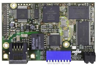
Figure 6-1: Ethernet / IP – Modbus TCP Option Board
