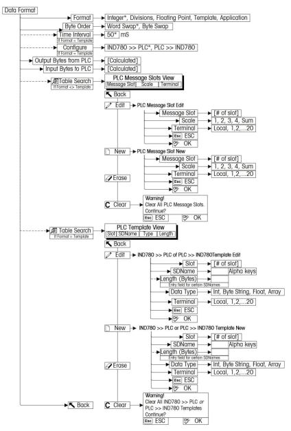
Figure 7-7: PLC Data Format Setup Block
