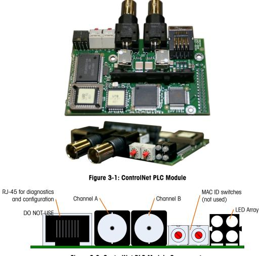
Figure 3-2: ControlNet PLC Module Components
