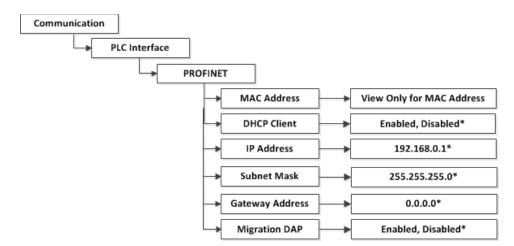
Figure 8-6: PROFINET Setup Block
