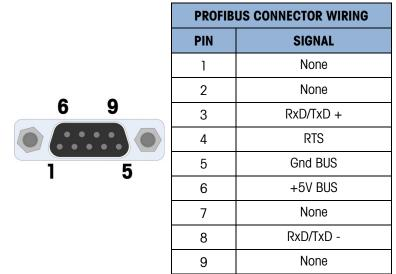
Figure 7-5: PROFIBUS Option Card DB-9 Connector Termination
