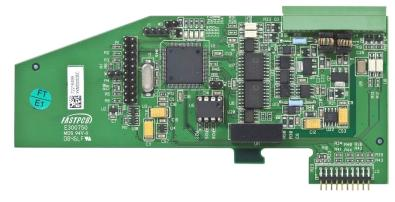
Figure 2-1: Analog Output Option Board
