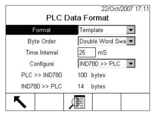
Figure 6-8: PLC Data Format Screen
