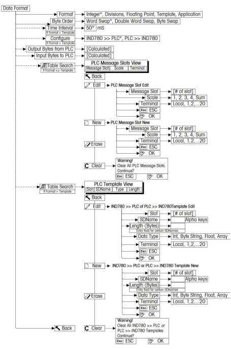
Figure 6-6: Modbus TCP Data Format Setup Blocks
