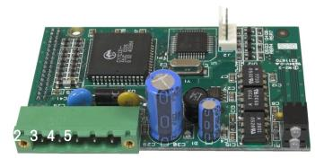
Figure 4-4: DeviceNet Connector Pin Numbering
