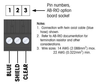
Figure 1-4: Three-Position Terminal Strip Wiring
