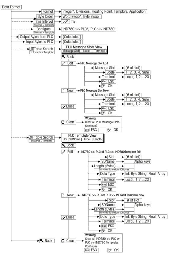
Figure 5-7: PLC Data Format Setup Block
