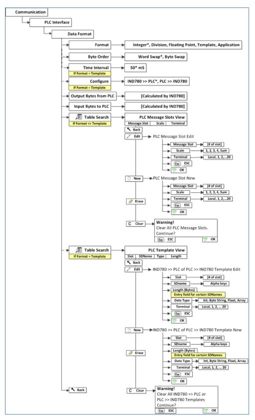
Figure 8-7: PLC Data Format Setup Block
