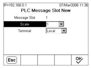
Figure 5-12: New Message Slot Screen
