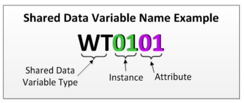
Figure 8-46: How a Shared Data Name is Constructed
