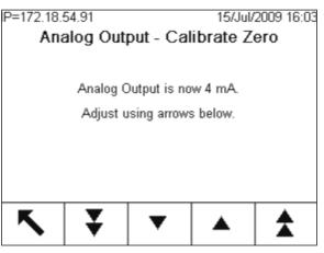
Figure 2-5: Analog Output – Calibrate Zero Screen
