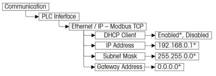
Figure 5-6: EtherNet / IP Setup Block
