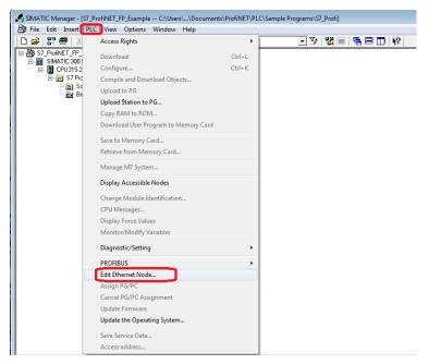
Figure 8-16: Configuration via DCP
