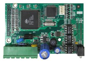
Figure 4-1: DeviceNet Option Board
