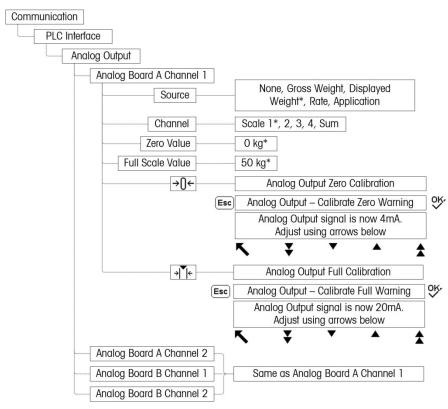
Figure 2-3: Setup Procedures for Configuring the Analog Output Option Card
