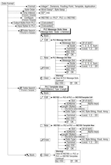
Figure 3-9: PLC Data Format Setup Block
