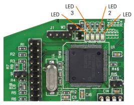
Figure 2-7: Analog Output LEDs
