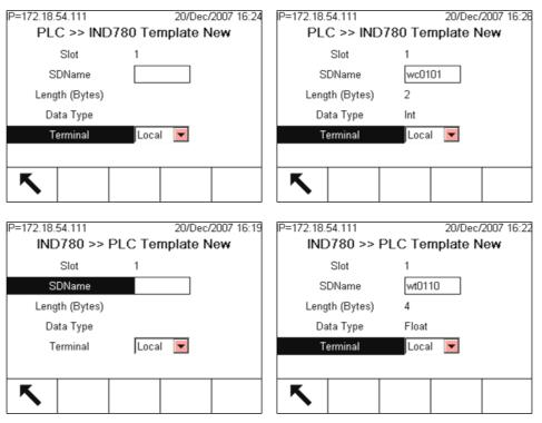
Figure 8-14: New Template Screens, PLC to IND780 and IND780 to PLC
