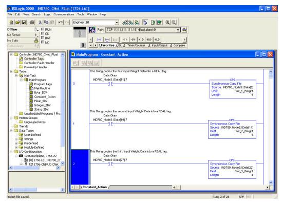
Figure 3-21: Float ControlNet 4-Slot Weight to Tag
