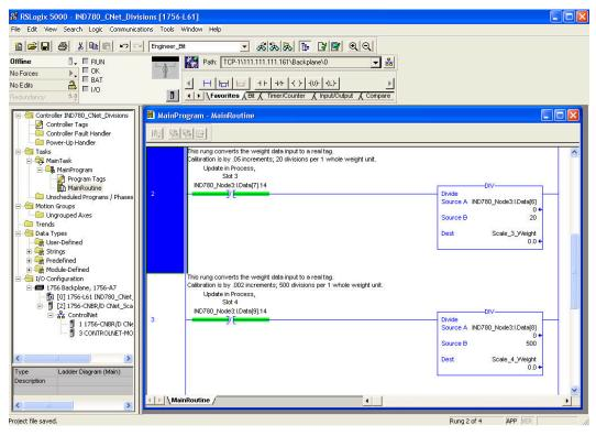
Figure 3-19: DIV ControlNet 4-Slot Weight 2 Tab Setup
