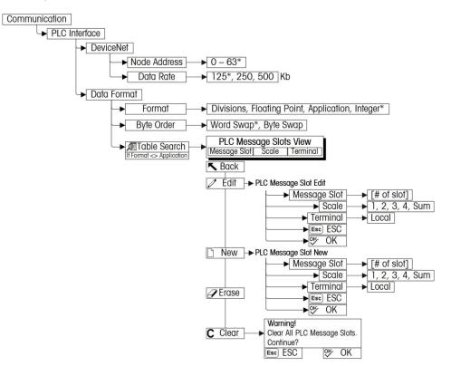
Figure 4-5: The DeviceNet Program Block and Data Format Setup Block
