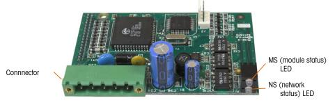
Figure 4-2: DeviceNet Option Board Components
