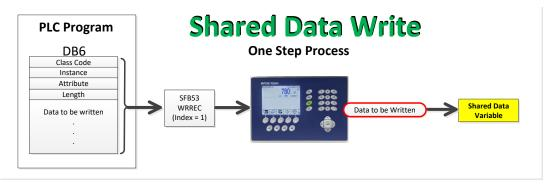
Figure 8-48: Shared Data Write – One Step Process
