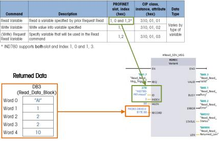
Figure 9-11: Instructing the Terminal to Send Data
