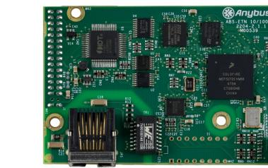
Figure 8-1: PROFINET Module
