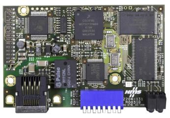
Figure 5-1: EtherNet / IP Module
