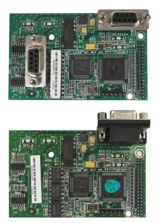
Figure 7-1: PROFIBUS Interface Module: Panel Mount (top) and Harsh (bottom)
