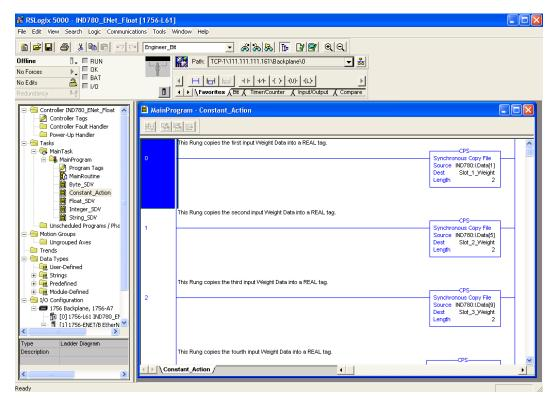
Figure 5-20: Input Weight Data to Real Tag
