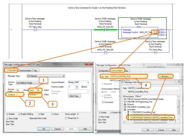
Figure 2-14: Ladder Logic – Taring the Scale
