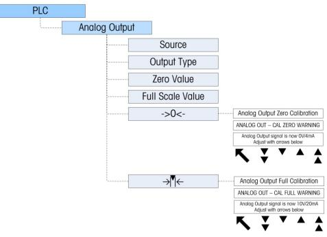
Figure 1-2 illustrates the setup procedures for configuring the Analog Output option for the IND570 terminal.
