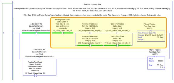
Figure 3-26: Filtering of Floating Point Data into PLC
