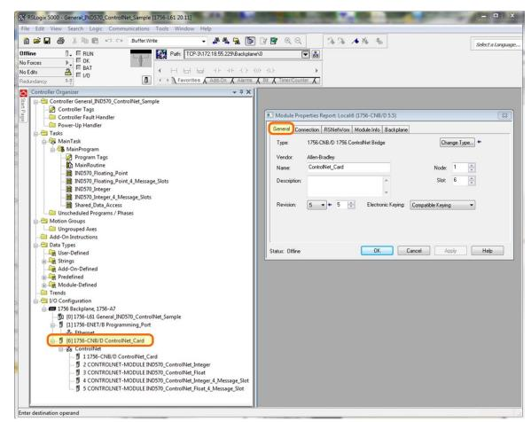
Figure 2-6 shows the configuration of the ControlNet Scanner Module (1756-CNB/D)
