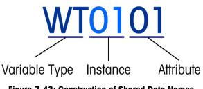
Figure 7-43: Construction of Shared Data Names
