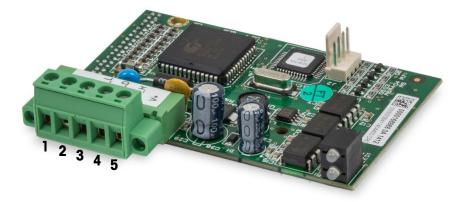
Figure 3-2: DeviceNet Connector Pin Numbering
