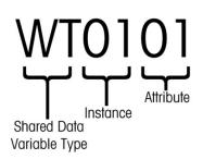
Figure 2-13: Construction of a Shared Data Variable Name
