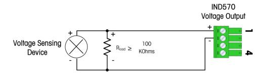
Figure 1-5: Typical Voltage Measurement Connection
