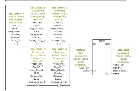
Figure 6-11: Filtering for Valid Data, Floating Point Mode
