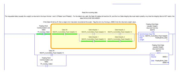
Figure 5-2: Correct Filter Ladder Logic for Floating Point Data
