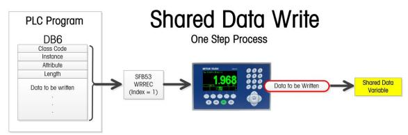
Figure 7-45: Shared Data Write – One Step Process
