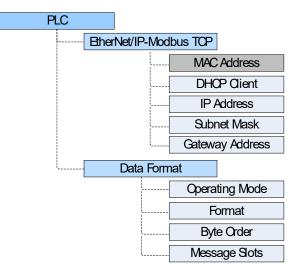
Figure 4-2: EtherNet/IP Setup Block
