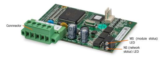
Figure 3-1: DeviceNet Option Board Components
