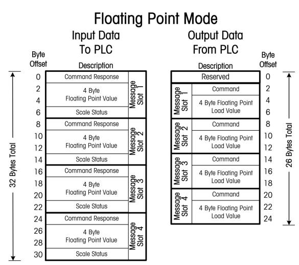
Figure 7-8 Floating Point Message Slot I/O Mapping
