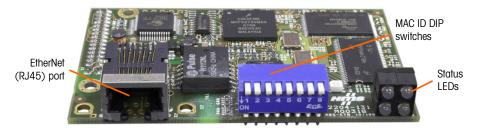
Figure 5-1: EtherNet/IP - Modbus TCP Option Board Components
