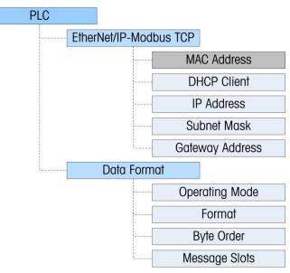
Figure 5-3: The Modbus TCP Setup Block
