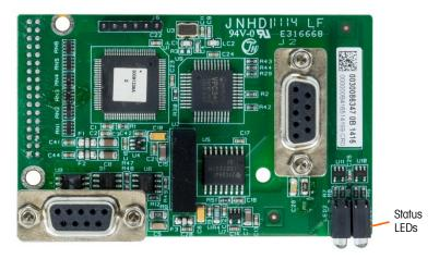
Figure 6-1: PROFIBUS Kit Option Board, Harsh Enclosure Version
