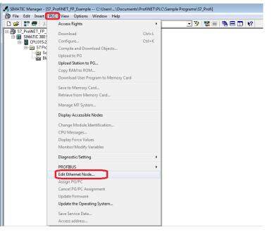
Figure 7-11: Configuration via DCP
