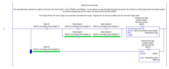
Figure 2-10: Filtering with Data\_OK Bit and Two Data Integrity Bits, Floating Point Mode
