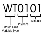
Figure 4-11: Construction of a Shared Data Variable Name
