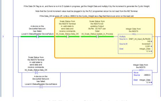
Figure 3-27: Filtering Integer/Divisions Data into the PLC
