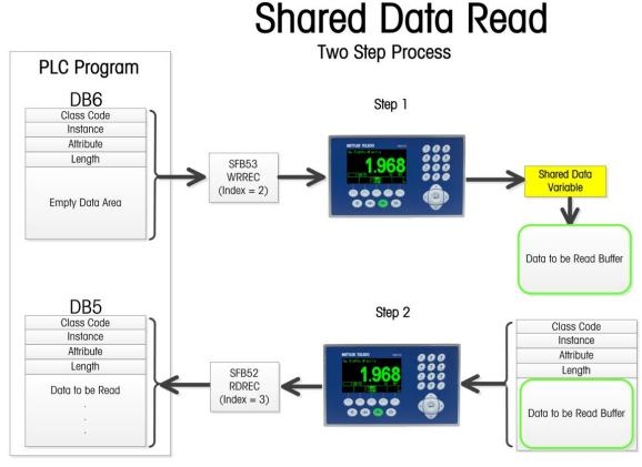
Figure 7-46: Shared Data Read – Two Step Process
