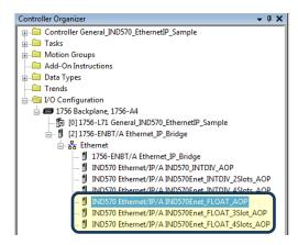
Figure 4-6: Floating Point Mode Sample Communication Module
