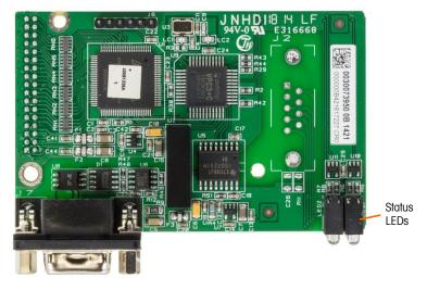
Figure 6-2: PROFIBUS Kit Option Board, Panel Mount Version
