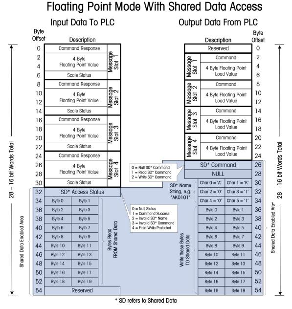
Figure 6-4: Floating Point I/O Mapping
