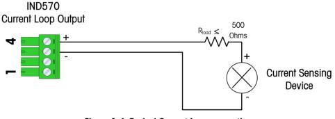
Figure 1-4: Typical Current Loop connection
