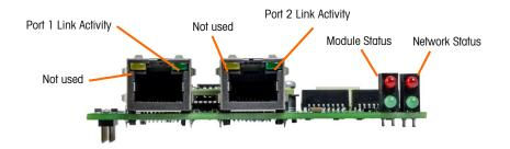
Figure 7-18: PROFINET Status Indicator LEDs
