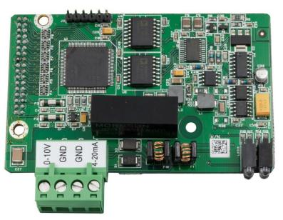
Figure 1-1: Analog Output Option Board
