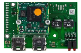
Figure 7-1: PROFINET Module
