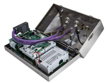
Figure 6-6: PROFIBUS Option Board Installed - Harsh Enclosure
