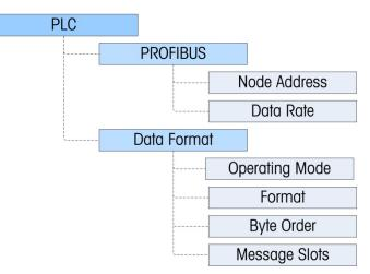
Figure 6-7: PROFIBUS Configuration Options in IND570 Setup
