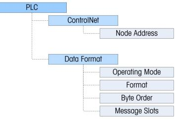
Figure 2-4: Setup Menu for ControlNet
