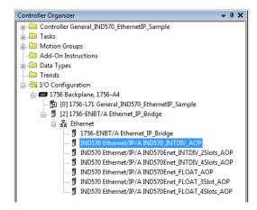
Figure 4-4: Integer Mode Sample Communication Module
