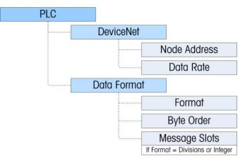
Figure 3-3: The DeviceNet Program Block and Data Format Setup Block
