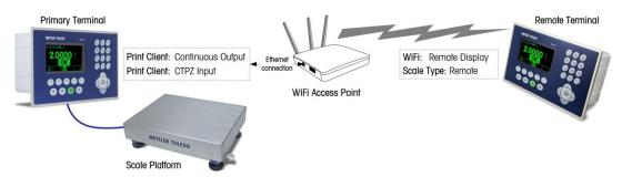
Figure 4-17: Example of Terminal Configuration for Remote Display Function via Wi-Fi
