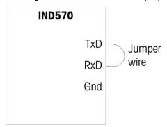
Figure 5-15: Jumper Wire Between Transmit and Receive Terminals
