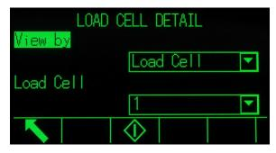
Figure 4-12: POWERCELL Load Cell Detail Selection Screen
