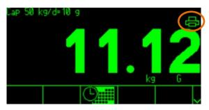
Figure C-5: Printer Connection Status in System Line
