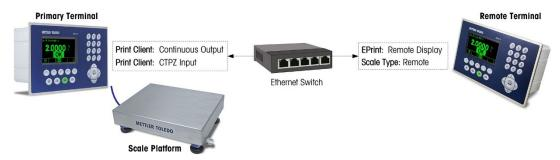
Figure 4-16: Example of Terminal Configuration for Remote Display Function via Ethernet
