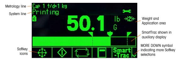
Figure 2-14: Default Home Screen, System Line with Print Message Displayed
