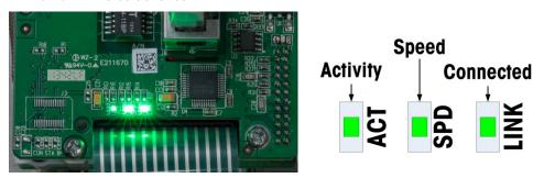
Figure 5-10: Ethernet TCP/IP LEDs
