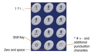
Figure 2-7: Alphanumeric Keypad Layout
