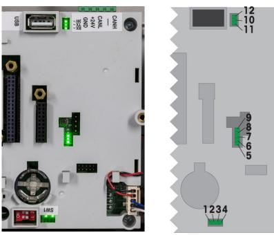
Figure 5-9: POWERCELL Main Board LEDs
