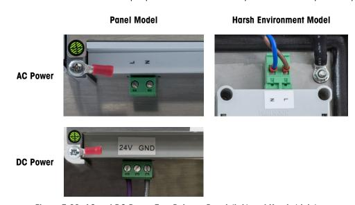
Figure 5-11: AC and DC Power Test Points – Panel (left) and Harsh (right)
