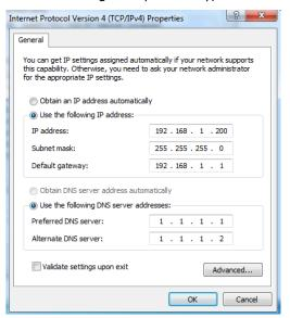
Figure C-3: Internet Protocol (TCP/IP) Properties Screen
