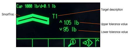
Figure 2-28: Over/Under Display, Large
