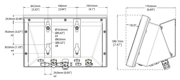
Figure 1-9: Harsh Environment Enclosure Dimensions with Fixed Angle Mounting Brackets for VESA
