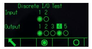
Figure 5-16: Discrete I/O Test Screen
