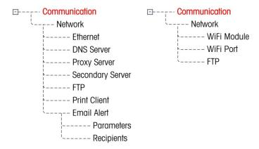
Figure 3-21: Ethernet TCP/IP Menu Structure (left) and Wi-Fi Menu Structure (right)
