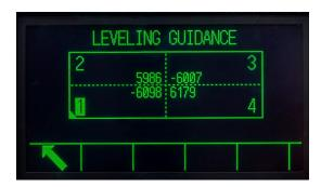
Figure 5-6: Leveling Guidance Graphic Display
