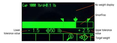
Figure 2-24: Material Transfer SmartTrac, Large
