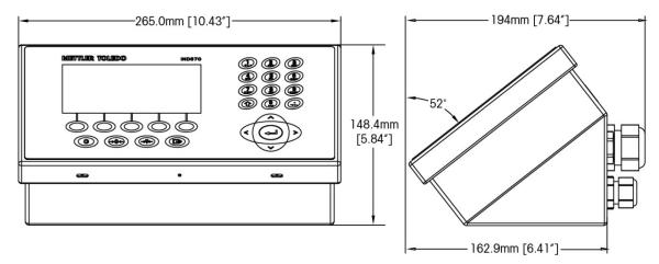
Figure 1-5: IND570 Harsh Environment Enclosure Dimensions
