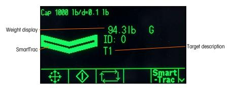
Figure 2-27: Over/Under Display, Medium
