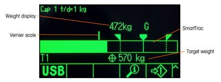
Figure 2-23: Material Transfer SmartTrac, Medium
