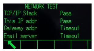
Figure 5-17: Network Test Screen
