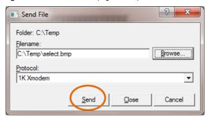
Figure C-8: Serial File Transfer Screen
