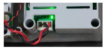
Figure 5-7: 12-VDC LED on Power Supply
