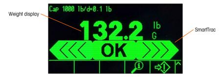
Figure 2-26: Over/Under Display, Small
