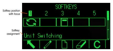
Figure 3-18: Softkeys Setup Screen
