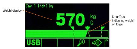
Figure 2-22: Material Transfer SmartTrac, Small
