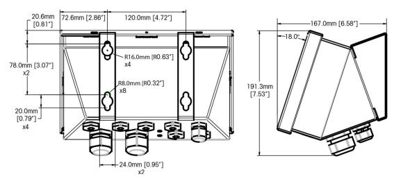
Figure 1-7: IND570 Harsh Environment Enclosure Dimensions with Fixed Angle Mounting Brackets,
