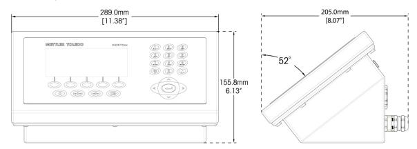
Figure 1-8: Harsh Environment Enclosure Dimensions, IND570xx
