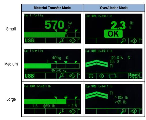
Figure 3-16: SmartTrac Display Sizes, Material Transfer and Over/Under Modes
