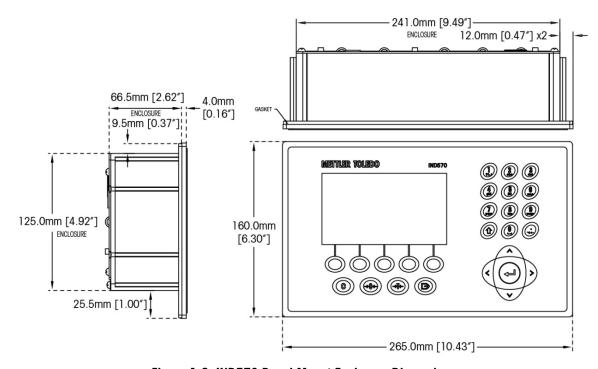
Figure 1-3: IND570 Panel Mount Enclosure Dimensions
