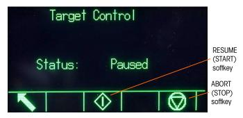
Figure 2-21: Example of Paused State in Target Control
