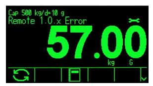
Figure 2-38: Asynchronous Error System Line Message
