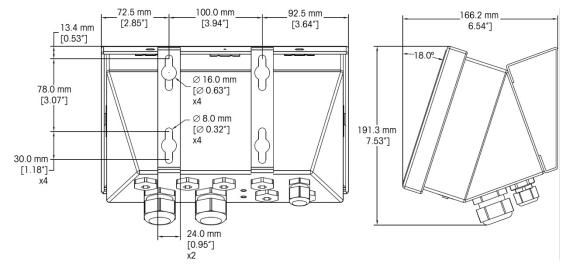
Figure 1-6: IND570 Harsh Environment Enclosure Dimensions with Fixed Angle Mounting Brackets, VESA
