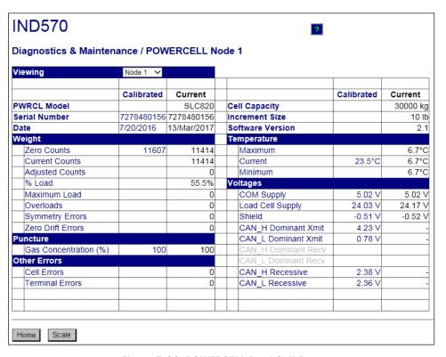
Figure 5-36: POWERCELL Load Cell Data
