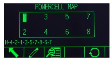
Figure 3-35: Completed POWERCELL Load Cell Map
