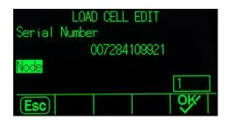
Figure 3-12: Manual Address Load Cell Edit Screen
