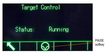
Figure 2-20: Example of Running State in Target Control
