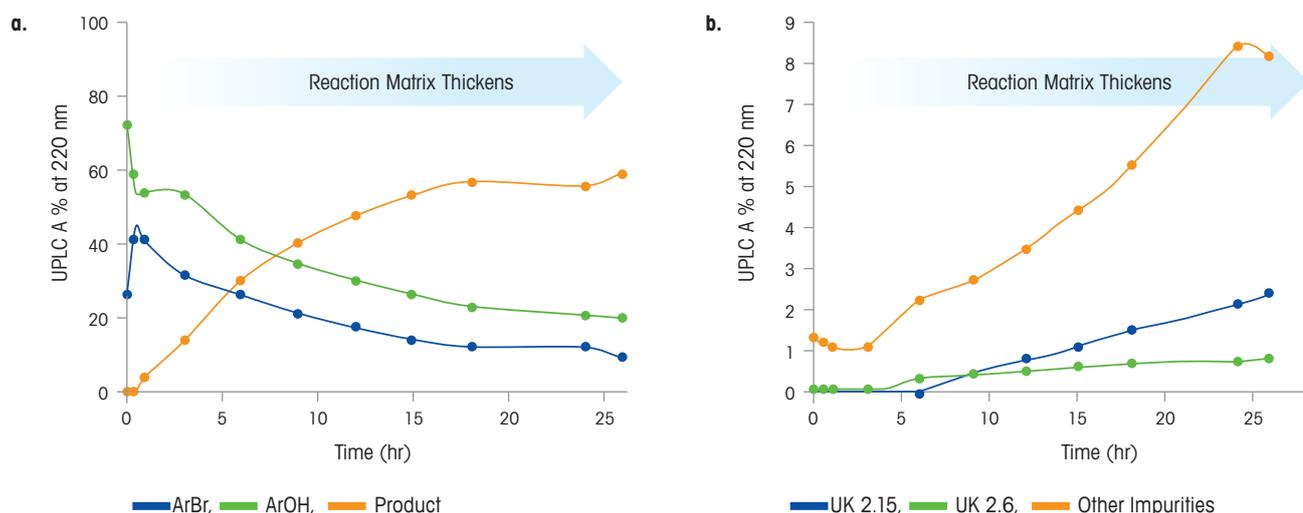
**Figure 2.** Progression of the Ullman reaction monitored by analysis of conversion (a) and impurity (b) profiles gained by UPLC analysis of representative samples acquired by EasySampler over 30 hours.
