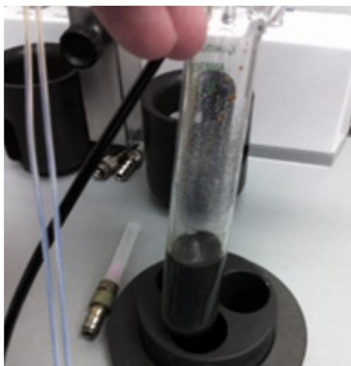
**Figure 1.** Dark Ullman reaction mixture in an EasyMax tube reactor
