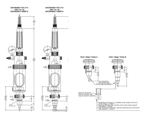
Different shapes for the lower part of the immersion tube.
