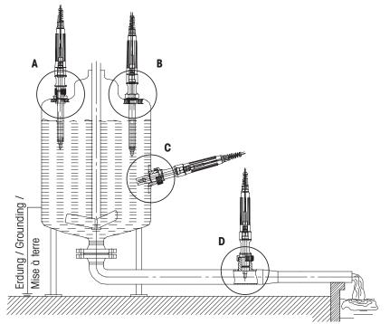
Connection of the housing to the potential equalization system of the plant.
