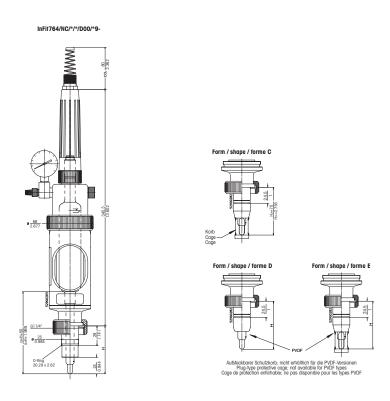
Different shapes for the lower part of the immersion tube.
