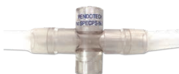
Flow Cell Installed with Tubing
