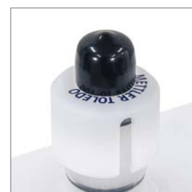
InSUS 607 installed in Eldon James weld-in bag port
