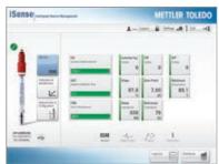
With iSense™ software, sensors can be calibrated via a PC or mobile device then connected to the M100 DR. Therefore, a user interface in the field is not necessary.
