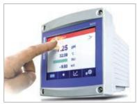
Touchscreen display provides simple, convenient operation, and any menu function can be reached in only three touches. Traffic light color coding means process or sensor issues are visible from a distance.
