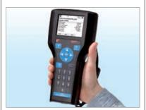
Access to ISM predictive diagnostic tools available over HART leads to reduced maintenance and increased process uptime.
