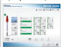
With iSense™, the key tool of ISM, sensors can be precalibrated via a PC then connected to the M100. Therefore, a user interface in the field is no longer necessary. This new transmitter concept reduces the operation and wiring effort to a minimum.
