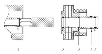
Flushing chamber (O-rings "2"): EPDM Ø17.86x2.62, FKM: Ø17.86x2.62, FFKM: Ø17.86x2.62
