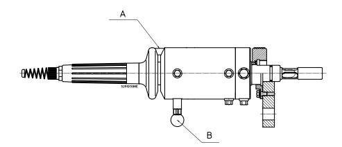
In the "Measuring" position, the immersion tube is fully inserted. The process medium flows past the tip of the electrode/sensor through the openings at the end of the immersion tube. O-rings seal the housing against ingress of process medium.
