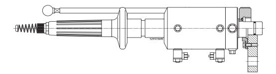
In the "Maintenance" position, compressed air pressurizes the immersion tube piston from below. In this position, the electrode/sensor can be cleaned or removed/exchanged, or the complete measuring system calibrated with the electrode/sensor installed. O-rings seal the housing against ingress of process medium. The housings are equipped with a pneumatic sensor detection system.
