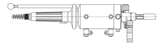
In the "Measuring" position, compressed air pressurizes the immersion tube piston from above. The process medium flows past the tip of the electrode/sensor through the openings at the end of the immersion tube. O-rings seal the housing against ingress of process medium.
