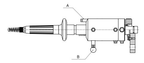
In the "Maintenance" position, the electrode/sensor can be cleaned or removed/exchanged, or the complete measuring system calibrated with the electrode/sensor installed. O-rings seal the housing against ingress of process medium.
