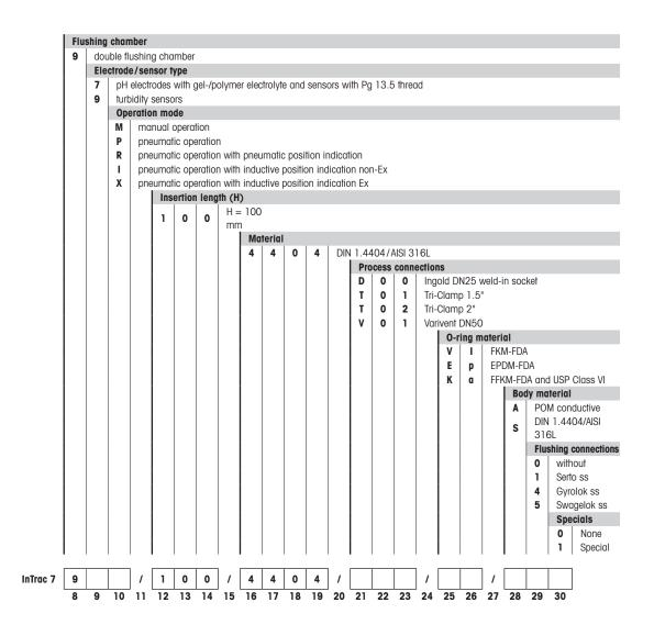
Housings with double flushing chamber are only available with DN25, Tri-Clamp or Varivent process connections. – Please contact your local METTLER TOLEDO representative for more options.
