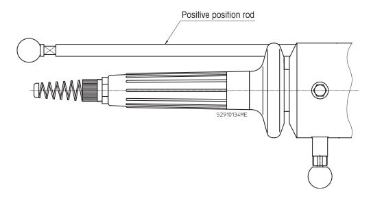
**Danger!** If the immersion tube comes to rest in an undefined position, this can lead to blockage of the inlet or outlet of the flushing chamber(s), and the flow of cleaning and flushing medium to the sensor will be impaired.
