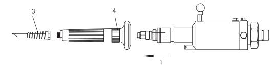
1. Move the housing into the "Maintenance" position.
