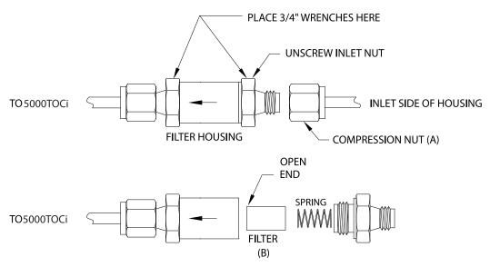
REPLACING THE FILTER ELEMENT FOR THE HIGH CAPACITY INLET FILTER
