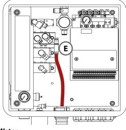
Connect the tube with the red marking to the compressed-air supply to media adapter (E) (located to the right of the control valves). This tube has a reduced connection diameter of 4 mm.
