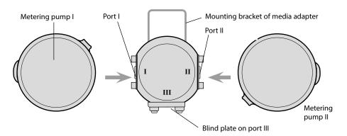
Top view of media adapter. The metering pumps are simply plugged on and fixed with two captive screws.
