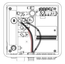
The tubes for water and purge air are identical. Connect one of the transparent tubes to the water control valve (B). Tighten the coupling nut hand tight. When you do not use air purging, connect the second transparent tube to the water control valve (B<sub>2</sub>). To do so, unscrew the sealing cap from the right outlet of
