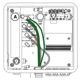
3. When the Aux 1 purge air control valve (C) is connected, unscrew the sealing cap and connect the second transparent tube here.
