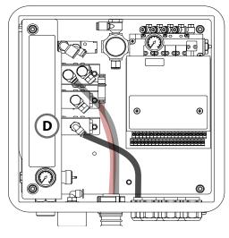
The tube for the optional Aux 2 control valve is not included in the media connection.
