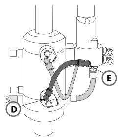
Feedback of "Process" position: Connect the "Process" feedback unit (D) of the probe – unlabeled connecting port – with the "Feedback Process" port (E) on the adapter by a flexible tube.
