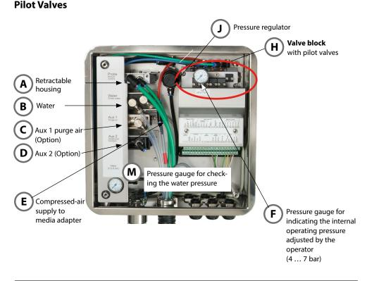
Pressure Gauges and Valve Block
