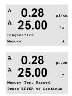
If Memory is selected then the transmitter will perform a RAM and ROM memory test. Test patterns will be written to and read from all RAM memory locations. The ROM checksum will be recalculated and compared to the value stored in the ROM.
