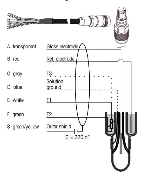
T1/T2: Temperature probe for 2-wire connection
