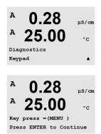
For keypad diagnostics, the display will indicate which key is pressed. Pressing [ENTER] will return the transmitter to the normal Measuring mode.
