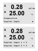
The digital Input menu shows the state of the digital inputs. Press [ENTER] to exit from this display.
