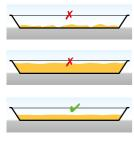
• Use the right sample volume. The pan should be thinly and evenly covered with the sample over the total surface area.
