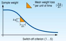
The switch-off criterion selected influences the measurement period and measurement accuracy. The drying process will be completed in the shortest time if AK 1 is selected, but the drying is then often not fully finished and repeatability is reduced. By selecting the switch-off criterion you optimize the duration of the measurement period against the required accuracy of the measurement result.
