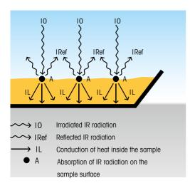
Different substances have different absorption characteristics. These depend primarily on the color and the material. You should therefore ensure that the sample is homogeneous and of even granulation. Smooth and light surfaces usually reflect infrared radiation more, so less energy is absorbed and the sample warms up less. This means that the absorption characteristics of a sample influence the effective sample temperature.
