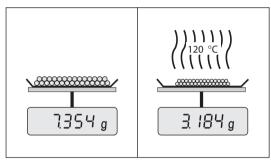
With halogen heating technology, maximum heating power is quickly reached and allows use of high temperatures. Uniform heating of the sample material ensures repeatability of the drying results and makes it possible to use small amounts of sample.
