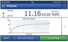
No color: Control and warning limits are not enabled. Note that the zoom function is also unavailable if no limits are set:
