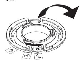
1 Turn the **draft shield lock** to the "" (Service) position.
