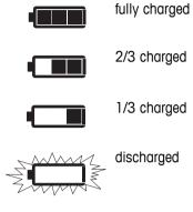
When the balance is operating on its batteries, the battery symbol in the display lights up. The number of segments that are lit is an indicator of battery condition (3 = fully charged, 0 = discharged). When the batteries are almost completely discharged, the battery symbol flashes.
