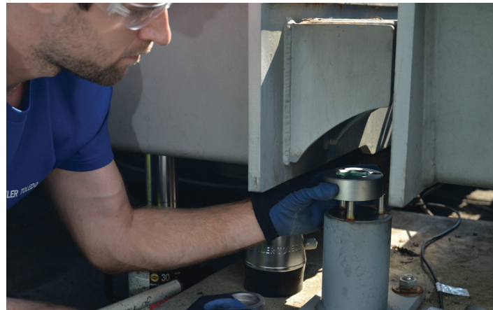
Periodically check load cells, receivers and other critical parts for wear
