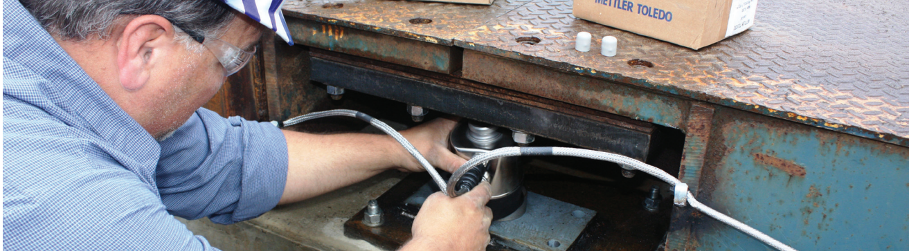
Upgrading an existing weighbridge by installing a new load cell system enhances the scale's accuracy and reliability
