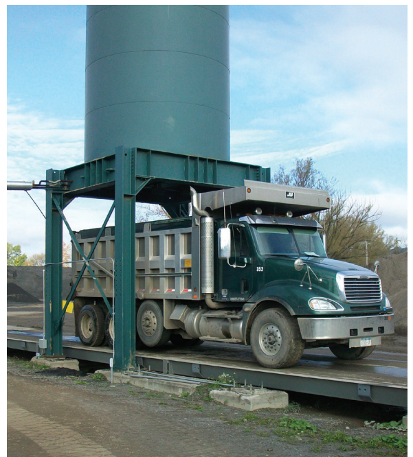
Filling operations may use a truck scale as the primary measurement for dispensing
