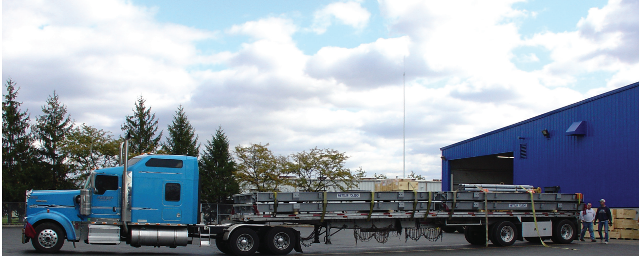
Transporting the weighbridge modules on a flat trailer is common in some places, although the width of the modules can mean that the truck requires an "oversized load" designation.
