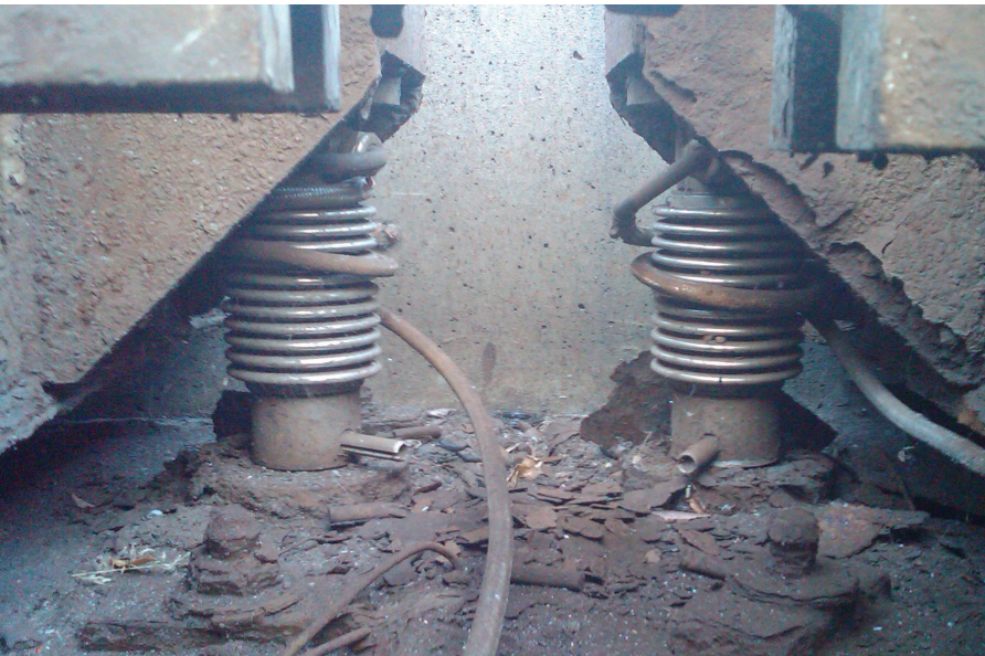
If a compression-style load cell has inadequate anti-rotation features, eventually the cable can wrap around the load cell and break.
