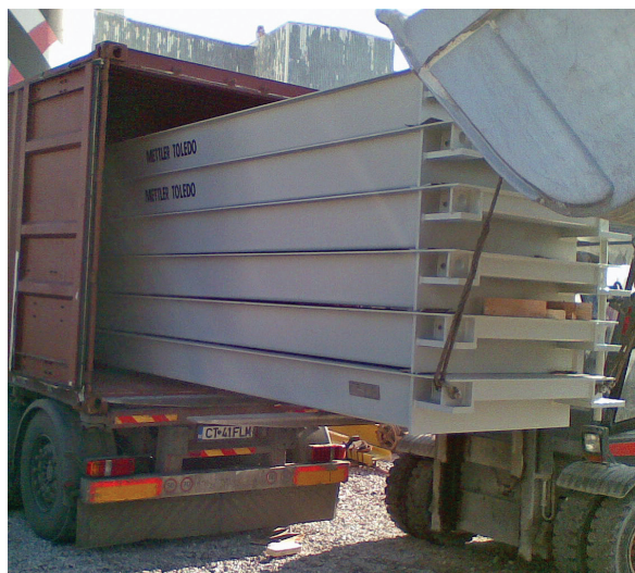
Some manufacturers can offer containerized scales to simplify transporting the scale long distances or to remote areas
