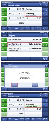
The EasySampler touchscreen shows the active sampling process.
