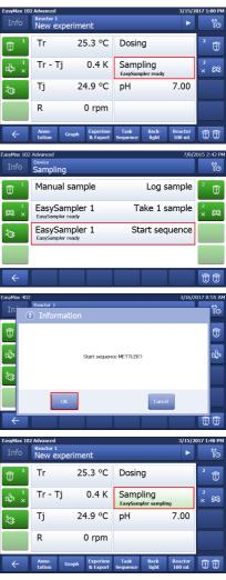
The EasySampler touchscreen shows the sampling sequence that is active.
