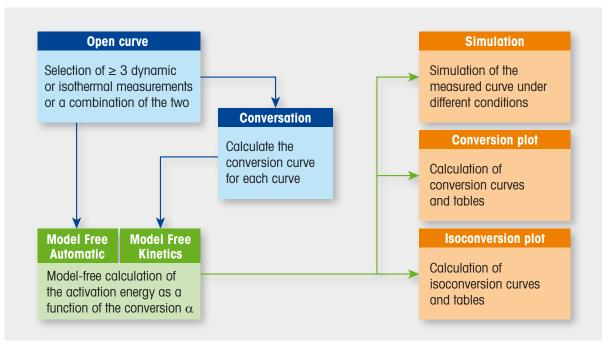
The possibilities offered by advanced MFK are ideal for the iterative improvement of predictions on the course of reactions if one wants to extrapolate over a large temperature range. Advanced MFK also allows the predictions of materials' long-term behavior to be significantly improved.
