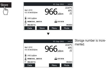
Note: automatic storage to memory can be switched on in the setup menu.
